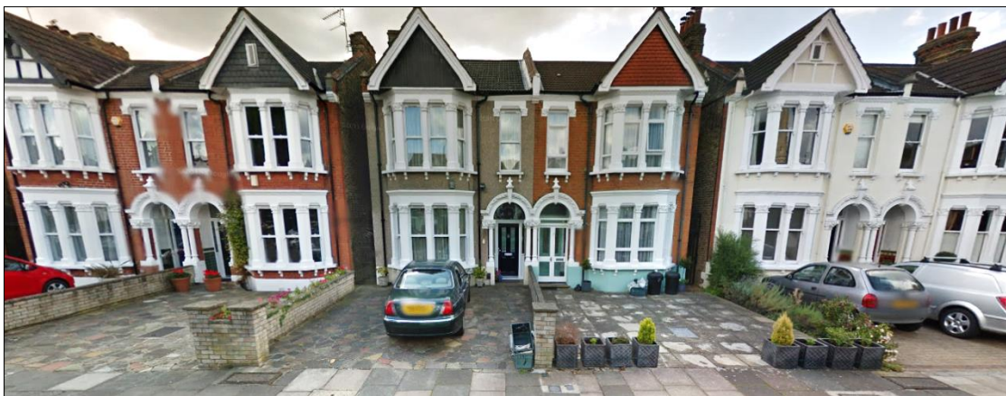
Figure 2: Domestic front gardens after vegetation has been replaced with hard impermeable surfacing to create off-street parking (Street View ©2015 Google)
