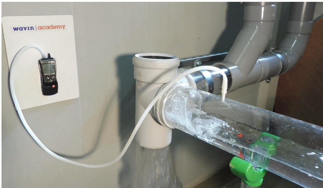
Figure 6 – Test 8. Double T 90°. Contamination 20%, water level 0.4.D. Mind the spectacular entrance of the water flow.
