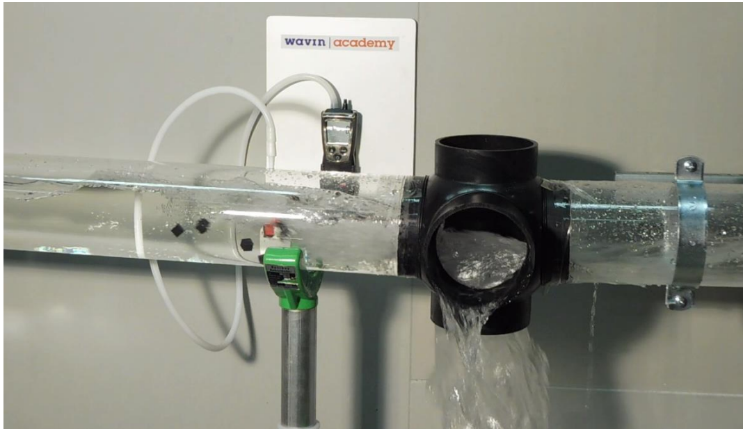
Figure 4 – Test 3, ball T 180°. Contamination 32%, water level 0.7.D
