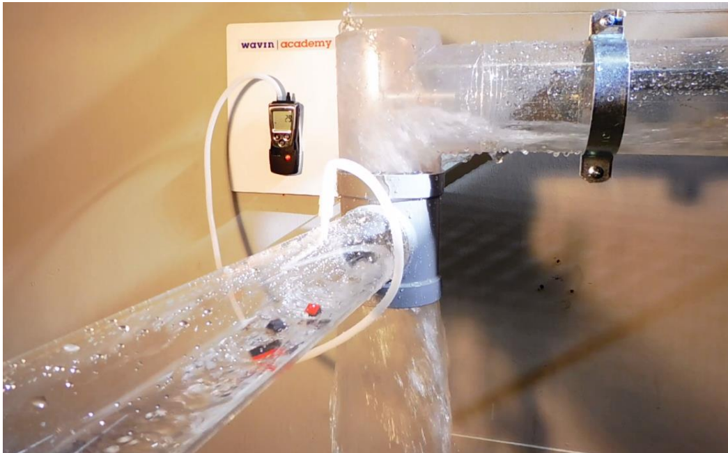
Figure 7 – Test 10. T at 90°. H = 150. Contamination 16%, water level 0.4.D
