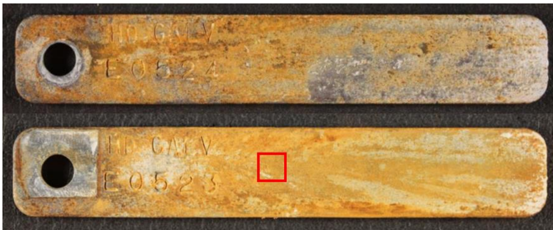
Figure 13 Coupons before Bifipro before cleaning. Top picture after 58 days, bottom picture after 127 days. Red spot indicates where sample for SEM/EDX was taken.
