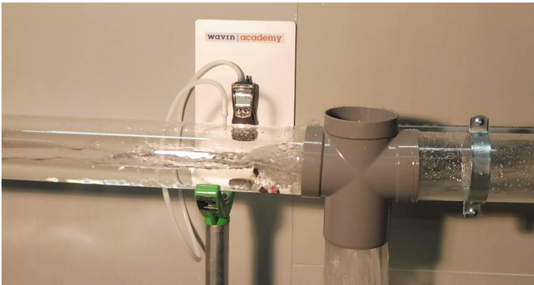
Figure 3 - Test 2, double T 180°. Contamination 40%, water level 0.4.D
